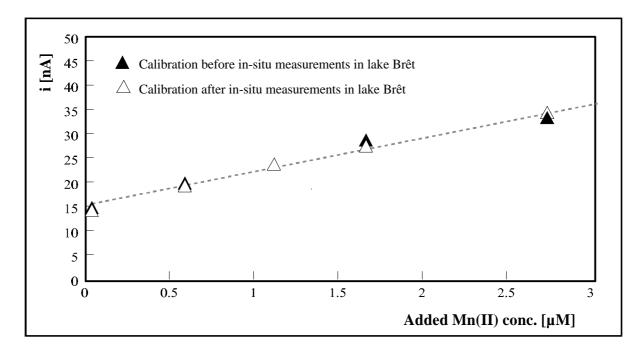
**Fig. 3 :** Typical SWASV results obtained for laboratory calibrations performed before and after in-situ measurements in lake Brêt using the same Hg layer over the three days.  $\mu$ -AMMIA Hg radius = 6.7  $\mu$ m. SWASV conditions : precleaning E= -800 mV ; precleaning t = 30 s. ; deposition E = -1600 mV ; deposition t = 10 s. ; final E = -1300 mV ; pulse amplitude = 25 mV ; step amplitude = 1 mV ; frequency = 5 Hz.
