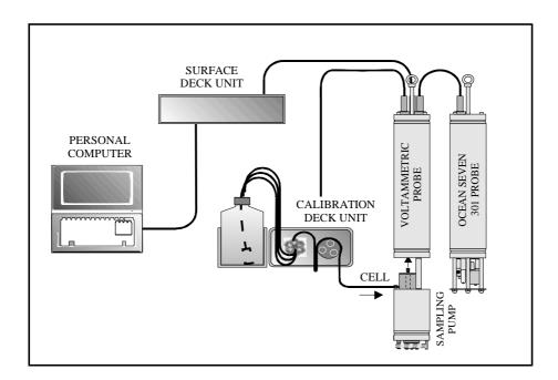
Fig. 1: Schematic diagram of the whole Voltammetric In-situ Profiling System (VIP System)
