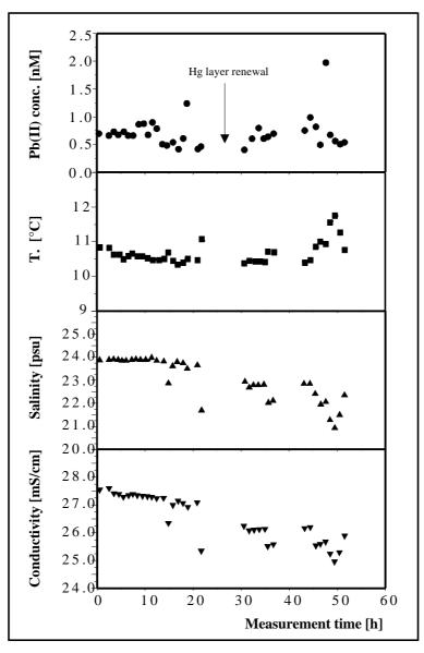
**Fig. 5 :** Unattended autonomous *in-situ* monitoring performed with the VIP System at Kristineberg Marine Station (Kullmar Fjord-Sweden May 16-18 1997).µ-AMMIE Hg radius = 8.3 µm. SWASV conditions : precleaning E = -80 mV; precleaning t = 60 s.; deposition E = -1300 mV; deposition t = 15 min; equilibration E = -1300 mV; equilibration t = 10 s.; final E = -80 mV; pulse amplitude = 25 mV; pulse step = 8 mV; frequency = 200 Hz.
